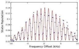
Figure 1: Ramsey fringes with a pulse gap of 0.8 ms. Total Raman power is around 8mW
